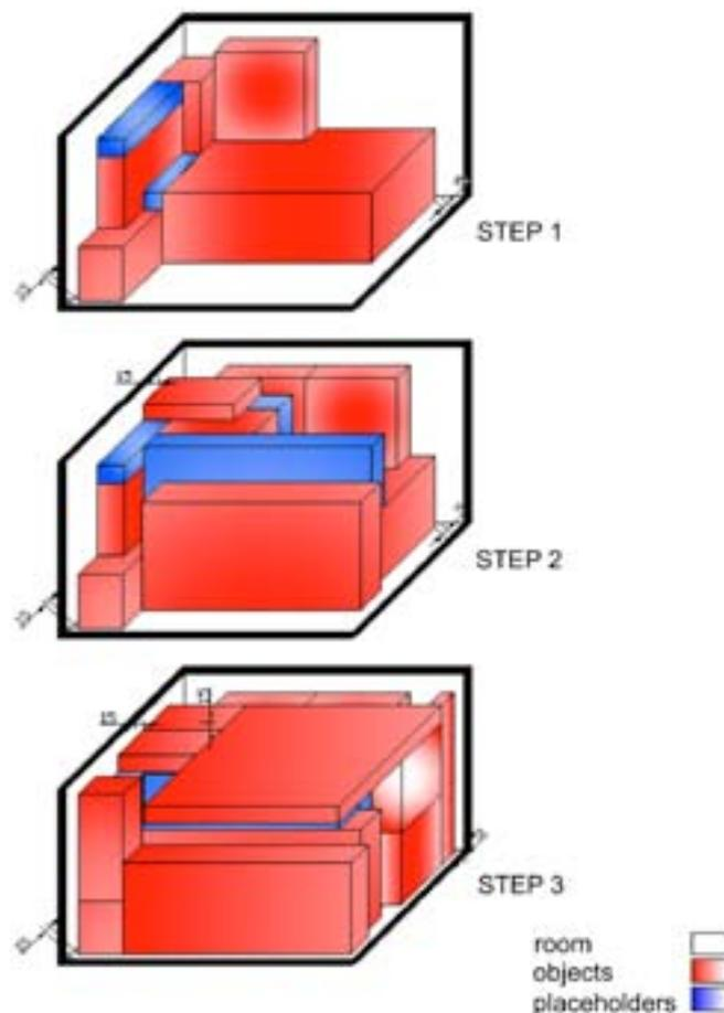
**Fig. 2:** Filling a shelter room in three steps
